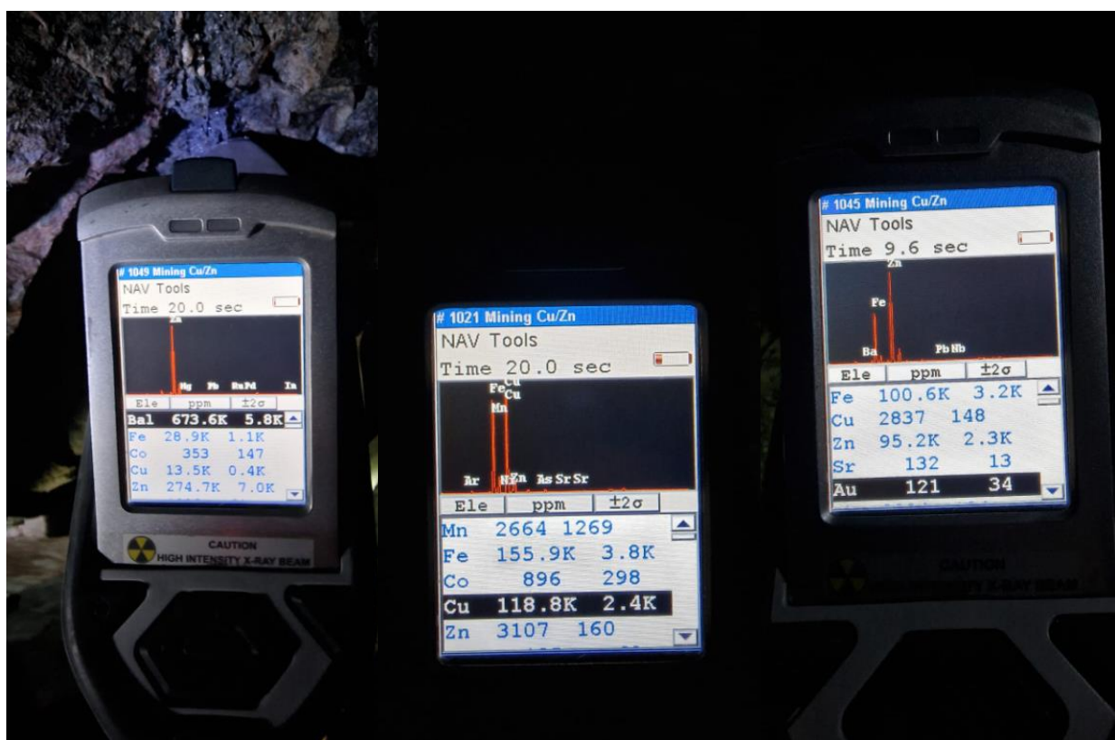
Figure 2: Screenshots of hand-held XRF-measurements from base metal mineralization on the walls of the Cu-Zn-Pb-Ag mineralized zone in G4. Grades are in ppm, which translates into 1.25 % Cu, 27.47 % Zn (left), 11.88 % Cu, 0.31 % Zn (middle), and 0.28 % Cu, 9.52 % Zn (right). Mineralization is accompanied by anomalous cobalt grades of 0.03-0.09 %.
